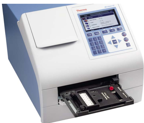
The \mu Drop Plate enables measuring low-sample volumes down to 2 \mu L and cuvettes
