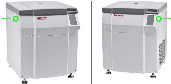
Figure V-2: Position of the mechanical emergency door release
